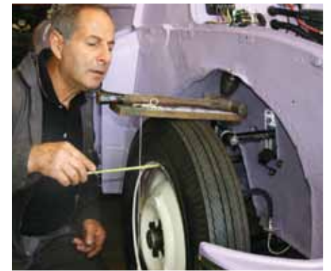
Percy is seen here manually working out the tracking by using a plumb-bob and strings.
