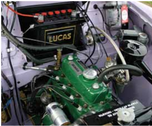
(below) the trusty 948 cc A series engine... reconditioned, polished and rearing to go!
