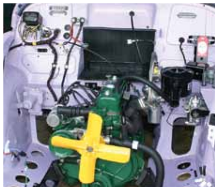
Wires were loosely put in place prior to final fitting to the electrical components.
